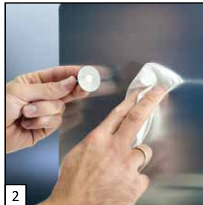
2 Clean fastener and substrate with scotchbrite and solvent
