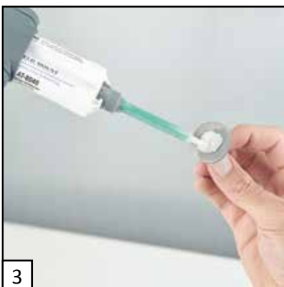
3 Squeeze the handle to dispense a small amount of adhesive onto the bottom of the part.
